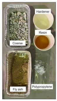
*Figure 2*. Materials used in the preparation of polymer concrete mixture
